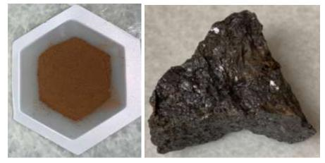
Figure 6. Ilmenite specimen from Fishersci (left) and Ward Scientific (right).
