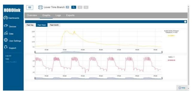
Figure 55. Screenshot of the graphed water level data and battery performance for the Lower Tims Branch HOBO data logger for a 1-week time period viewed through the HOBOlink website. Graphs can be generated for recorded data on a daily, weekly or monthly basis.
