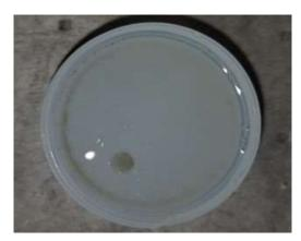
Figure 22. Suspension of white solid observed inside reactor from SPFT experiment at 70°C. The circle in the bottom left indicates where the suspension has held shape from the presence of the tubing.
