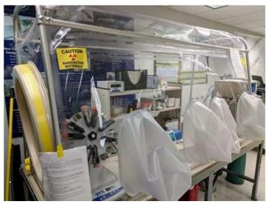
Figure 7. Anaerobic glovebox with 98% N<sub>2</sub>: 2% H<sub>2</sub> atmosphere where pertechnetate reduction experiments are currently taking place.
